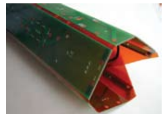
Flexible circuits are manufacturable in several layers.
