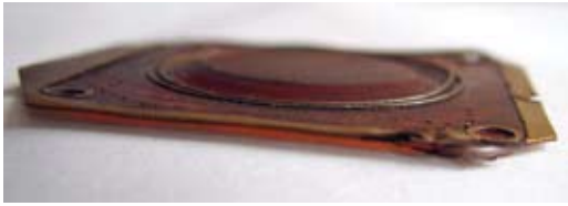
A double-sided circuit place copper on both sides of a dielectric layer.
