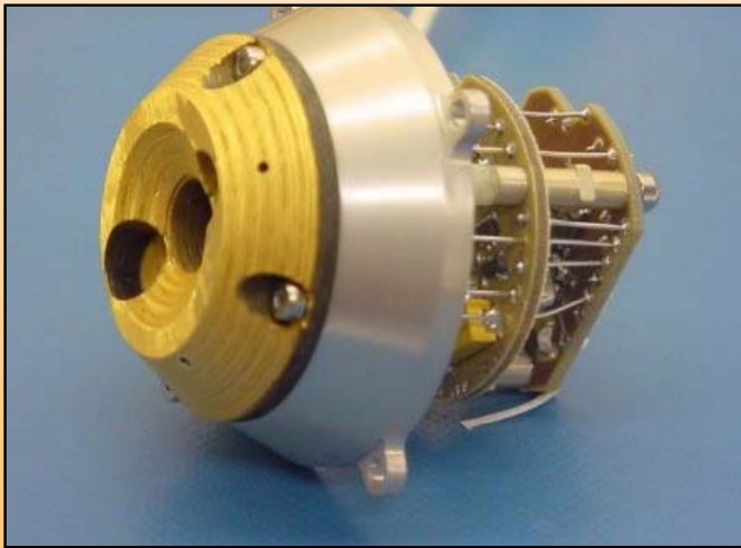
▲ X-Ray Spectrometer with cover to measure the elements in rocks
