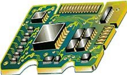
The use of heavy metal backplanes, thermal vias, thermal coins, heat spreaders, heat risers, and conductive adhesives are all proven ways in which materials can be used to reduce junction temperatures. Additionally, active cooling and water-cooling are also effective. Any or all of these methods can, however, adversely affect the cost, size, weight, reliability, and electrical performance of RF circuits.
